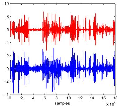
Figure 5: Signal level estimation of angular velocity using the magnetic field sensor vs. the gyroscope. To magnetic field sensor estimation is shifted by six units to make it easier to compare the two signals.
