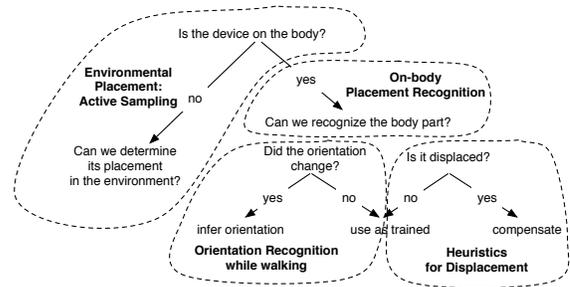
Figure 4: Categorization and contributions dealing with on-body placement effects of single sensing devices (Kunze 2011).
