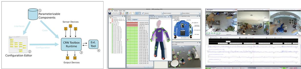
Figure 2: The Context Recognition Network toolbox concept on the left shows a repository of combinable components. The monitoring tool in the middle helps to keep track of sensor failures etc. during recordings. The labeling tool on the right helps to assign context labels and readjust sensor data in post-processing. All software is made available as open source (Bannach and Lukowicz 2011).
