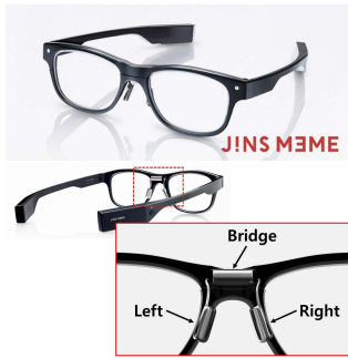
Figure 2: MEME: smart glasses with 3 electrodes to measure eye movements.
